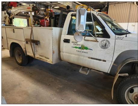
The 2002 Chevy Service Truck is still functioning, but note the "2x4 and ratchet strap band-aid" used to keep the doors closed.
